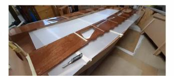
A dry fix run just to make sure all is ready. Back side of the panels all epoxied before fixing into position. Where the panels join the bulkheads its best to leave the
