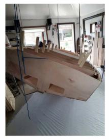
Before gluing the floor into position the floor bearer positions need to be marked on the insides of the hull ready for the side tank bulkheads as these must sit directly above the floor bearers.
