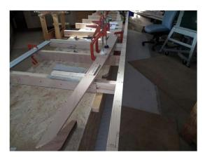
drawings. Check with the Kit supplier for any deviations in positions of bulkheads. You also need the set of measurements given to the kit supplier when his boat was first measured by the GP14 Association.
