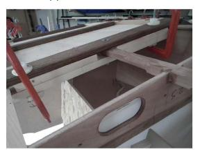
This is done in preparation for fixing the forward bottom sheet at the scarf joint and so making sure this joint is tight when glued.
