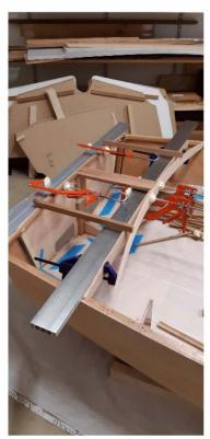
Rear deck beam, king plank and stringers ready for fixing. Notice the side tank panels not yet fixed as easier to work out position of rear curved beam and then cut slots in side tank panels. Slots need to be neat as these are the rear buoyancy tanks. Care is also taken to ensure all regulations are adhered to regards deck widths and depths.
